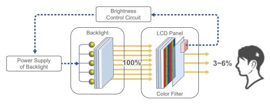
Figure 2. LCD Panel Construction Details
