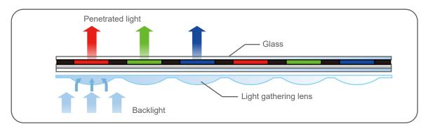
Figure 6. Diagram of light condensing lenses
